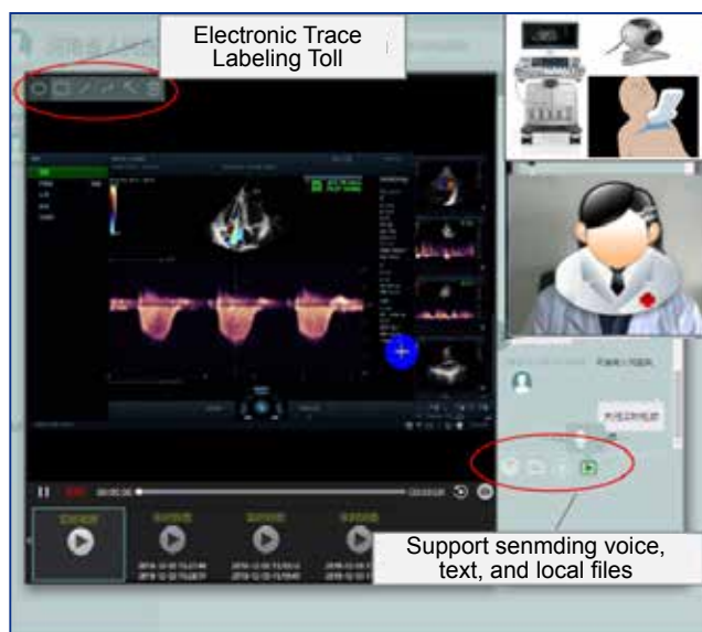
Figure 2 Consultation image of remote echocardiography based on cloud service. During the consultation, voice, video and ultrasonic images are transmitted simultaneously, and the two sides can communicate in real time.
