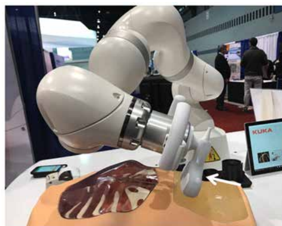
Figure 14 A light-weight six-axis robot system (Kuka, Augsburg, Germany) is depicted with the capability to maneuver and stabilize an ultrasound probe (arrow).
