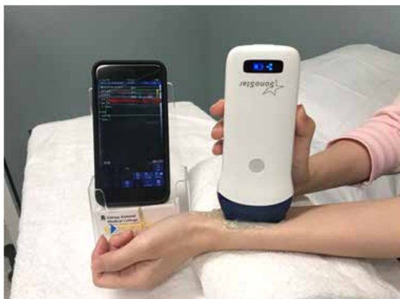
Figure 12 Handheld ultrasound unit is depicted (Sonostar Technologies Co., Ltd, Guangzhou, China). A wireless connection to a nearby smartphone is maintained for image visualization.
