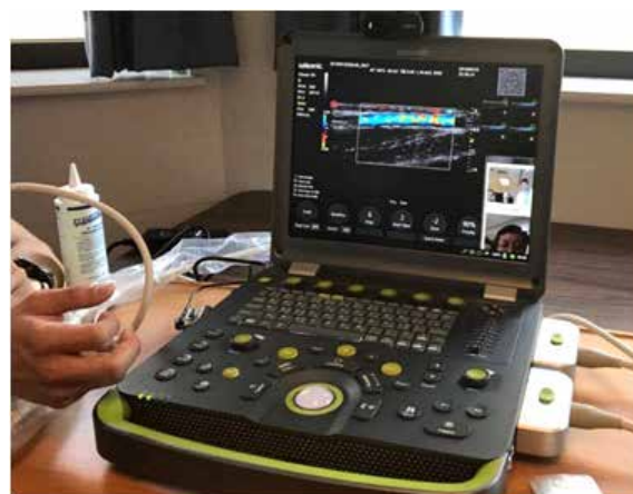
Figure 13 A portable ultrasound system (Shenzhen Wisonic Medical Technology Co., Ltd., Shenzhen, China) is depicted. The system utilizes a built-in telecommunication capability for real-time consultation for both domestic and international applications.
